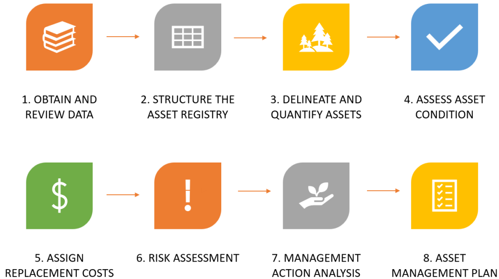
Figure 11-1. Overview of steps associated with natural asset management for Quartz Creek Community Watershed.
