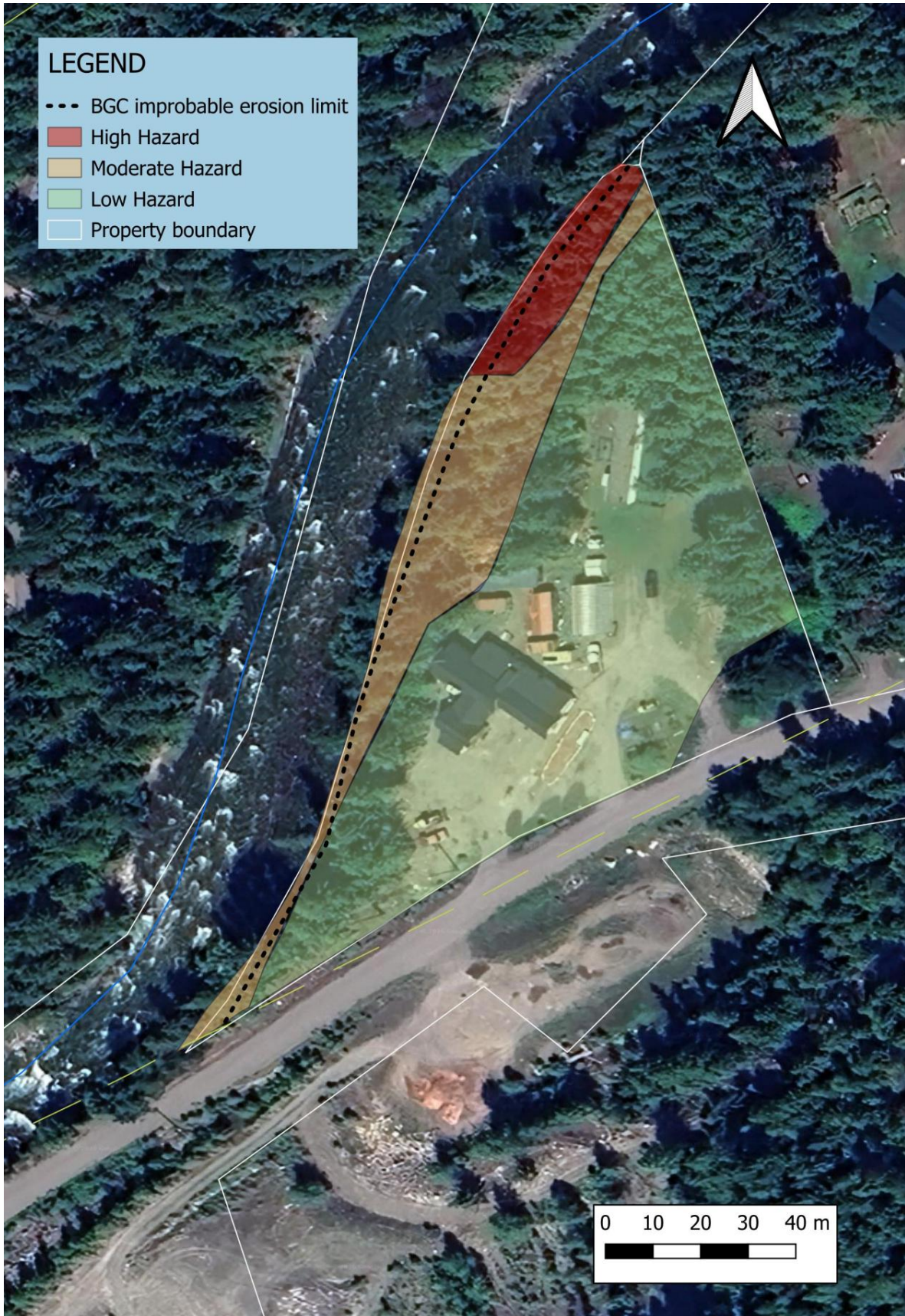
Figure 7. Figure showing erosion line and hazard areas from BGC report.
