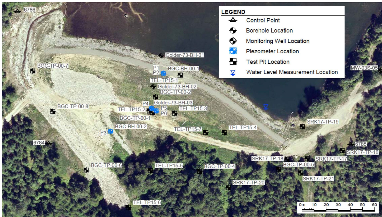
Figure 5: Locations of Historical Boreholes and Test Pits (2019 Dam Zones Review by SRK)
