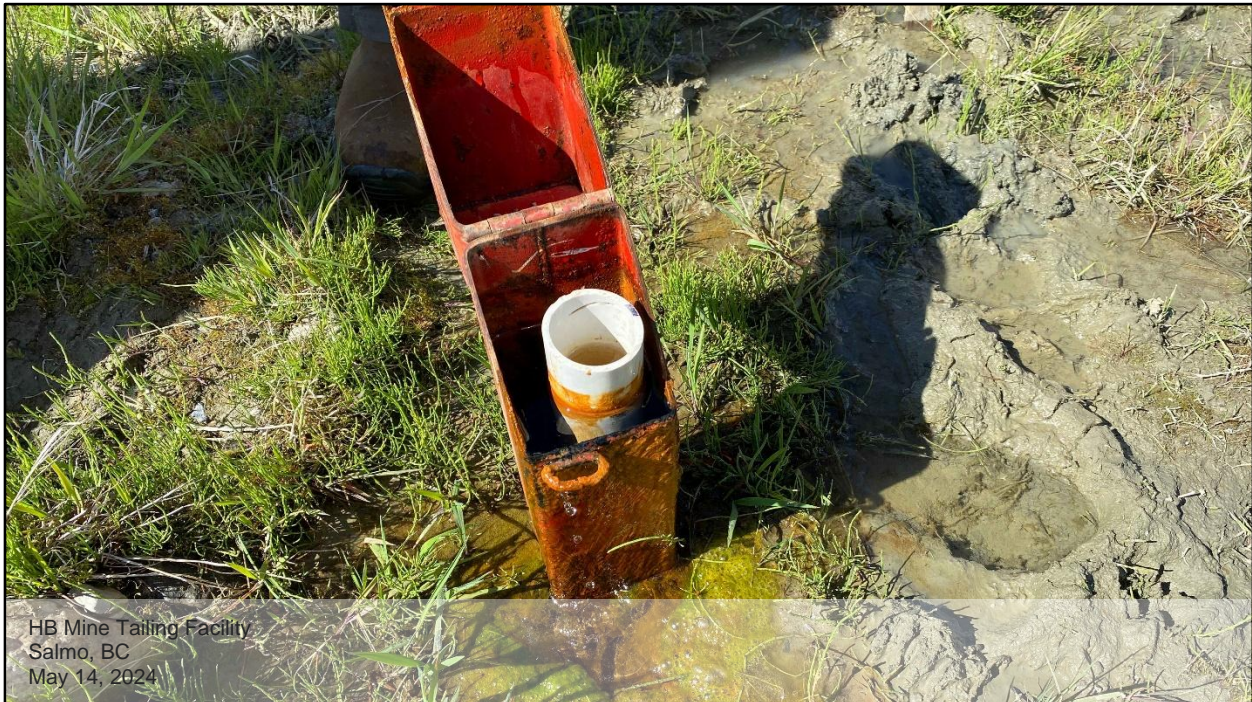
Photo D.31: A close view of the monitoring well MW-04-S-05 located in the tailing impoundment area. The pipe of the monitoring well was broken and found to be in flowing artesian condition.
