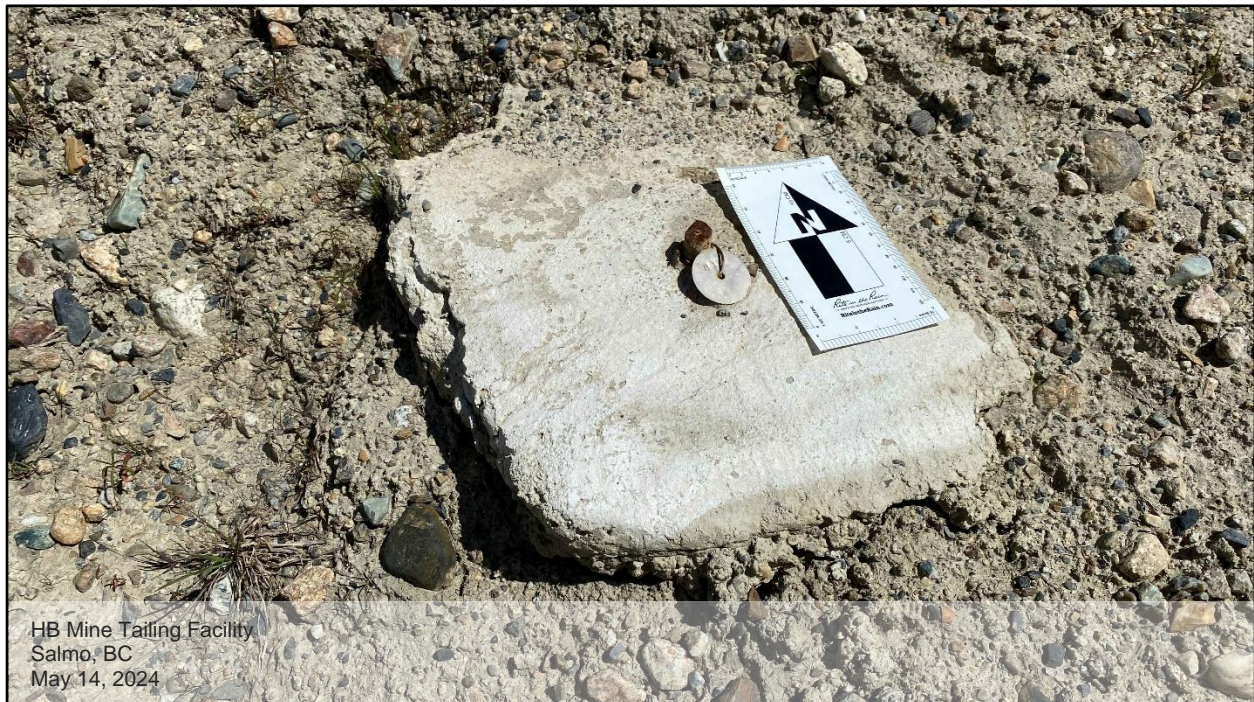
Photo D.20: A close view of the survey hub H11, located at the downstream slope of the expanded berm.
