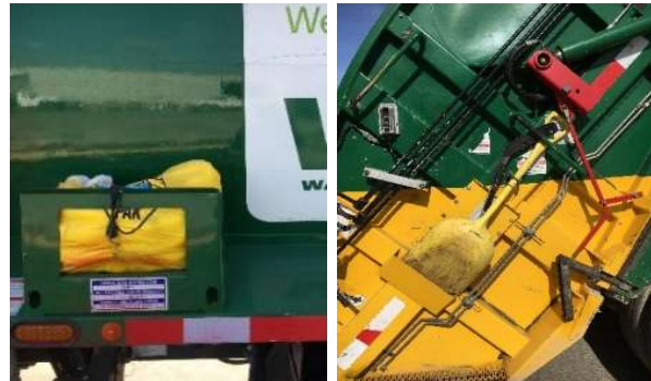
WM trucks have an onboard spill kit and shovel should a spill occur.
