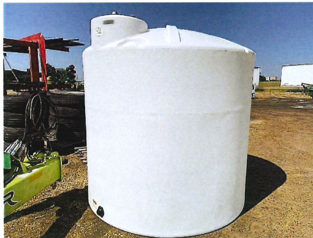
Figure 4:6000 USG vertical tank, to be housed in skidded enclosure with all pumps, reels, hose internal with a small heater.
